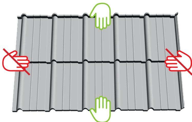
**Moving the sheets:** The sheets should be carried by their ribbings (green). It is not allowed to move the sheets by their edges (red), as it may cause gaps in the longitudinal overlaps.
