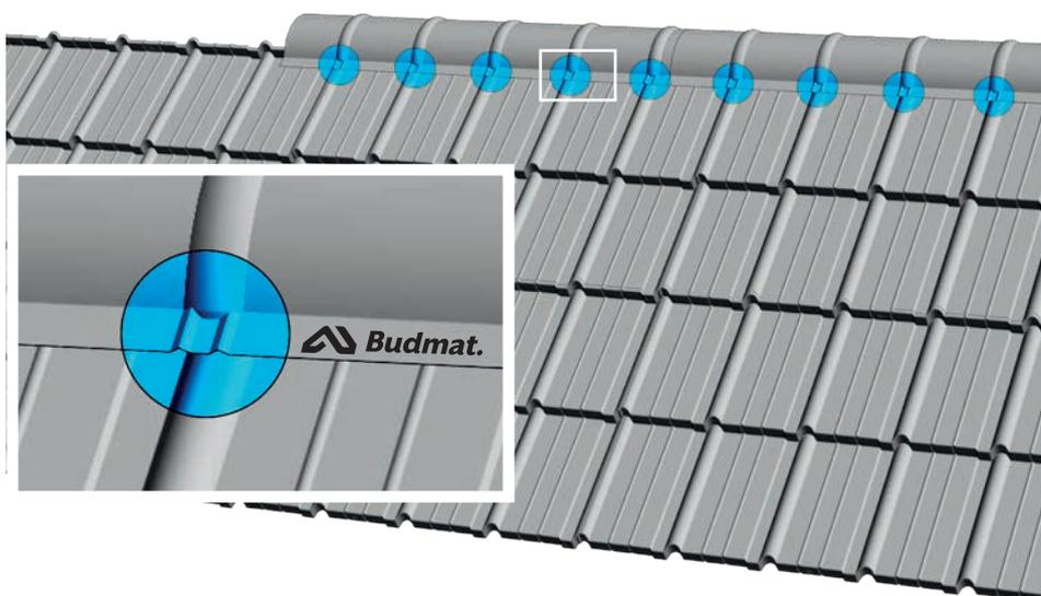
The ribbings of the ridge tile should flush with the highest points of the Murano modular roof tile sheet.
