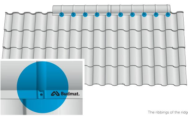
The ribbings of the ridge tile should flush with the highest points of the Rialto modular roof tile sheet. Embossed logo is a confirmation
